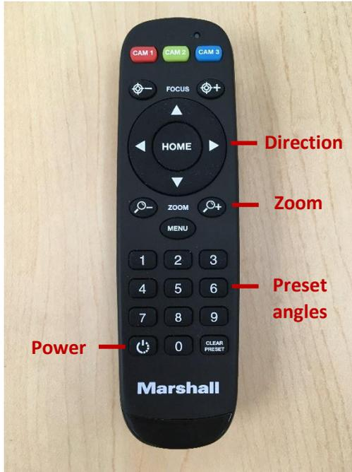
2. Use the arrow buttons (up, down, left, right) to adjust the direction of the camera.
